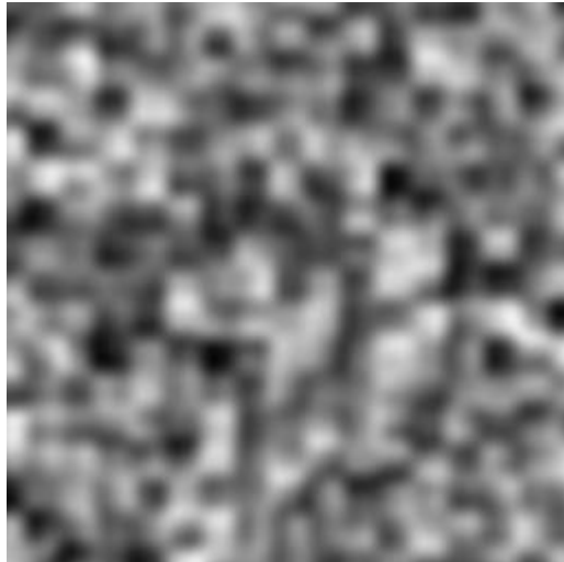
Figure 5.8.5: glm::perlin(glm::vec3(x / 16.f, y / 16.f, 0.5f));
